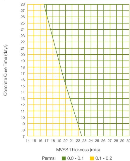
Green indicates Class I Vapor Diffusion Retarder capability as predicted by the test model. Minimum coating film thickness for obtaining the Class I rating depends on the specific field application conditions.
